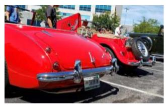
The BMC cars shared parts bins. The MG TD owner noticed the overriders on the rear bumpers of the TD and the 3000 were the same.
