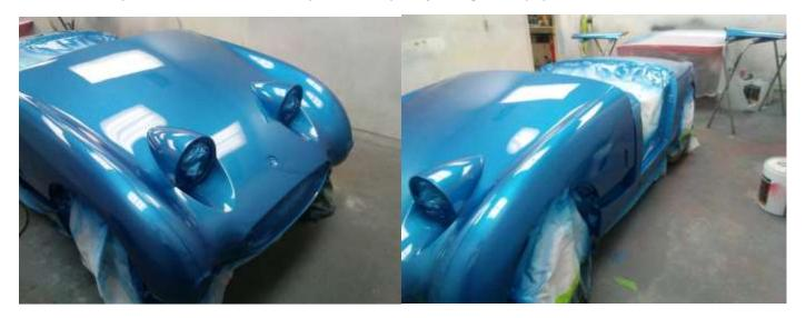
The paint still needs wet sanded/polished and they are also doing some touch up of the inside of the bonnet, inner fenders, and firewall.
