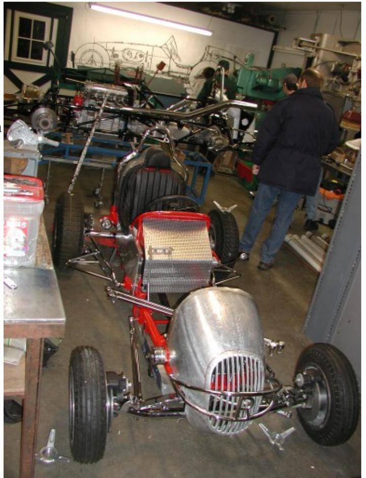
An original 289 AC Cobra body undergoing restoration at Hammer Art. The SuMar Indy car chassis is in the background. See the drawing on the wall.
