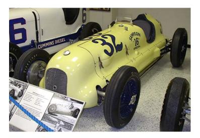
**Left:** Entered and built by Sampson Motors, this Stevens chassis was driven to 6th place in 1940 by Bob Swanson. *I could have had a V-8*! But it's engine, in fact, was a 183 cu in V-16, made by putting together (2) 91.5 cu in 8-cyl Millers in the form of a "V" over a common bottom end and crankshaft. 1956 winner Sam Hanks also drove it in 1946.
